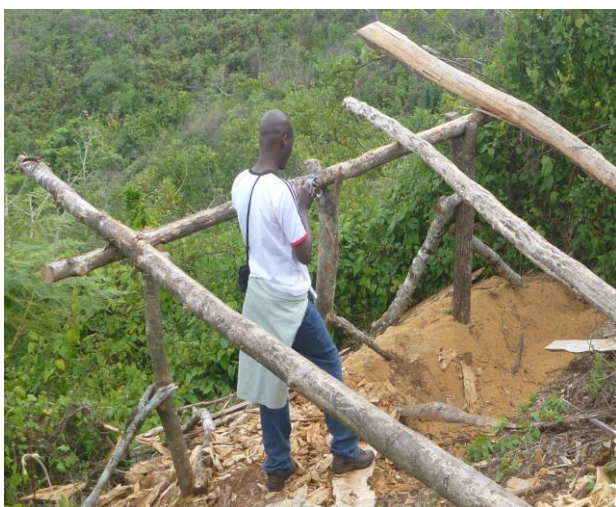
Small sized round wood of less than 10 cm being loaded for pit sawing on Zomba-Malosa Plateau
